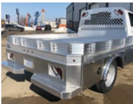
DROP-IN SIDES 6 1/2" extruded drop-in sides
